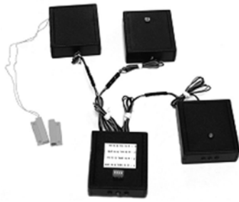
Figure 5: Garage Door Open At Night System built using eBlock prototypes.
