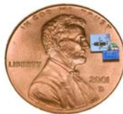
Figure 1: Approximate size of “Smart Dust” sensor nodes (photo courtesy of Joe Kahn).
