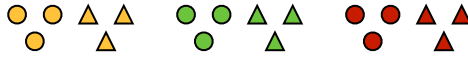
Figure 2. Representation of eighteen channels in a link having three fibers, three wavelengths per fiber, and two time slots per wavelength. Shapes represent time slots, shades represent wavelengths, number of shapes of a certain shade represents the number fibers.
