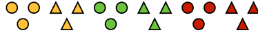
Figure 2. Representation of eighteen channels in a link having three fibers, three wavelengths per fiber, and two time slots per wavelength. Shapes represent time slots, shades represent wavelengths, number of shapes of a certain shade represents the number fibers.
