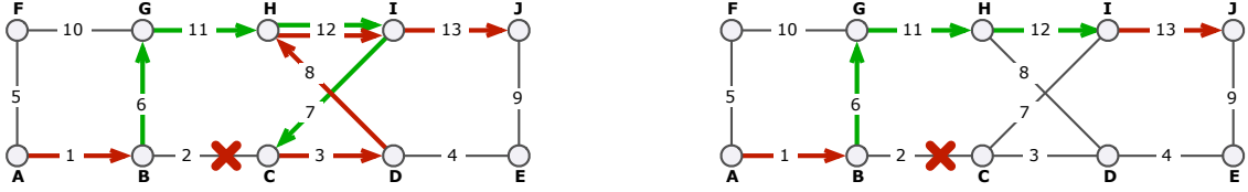
(c) Connection after failure of link 2 routed along 1–6–11–12–7–3–8–12–13.
