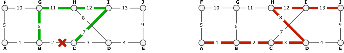
(a) Link 2 protected by backup path 6–11–12–7. (b) Primary path of a connection along 1–2–3–8–12–13.
